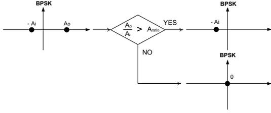
Fig. 3. Proposed Negative-Code-Collision Control Scheme in OCHM
