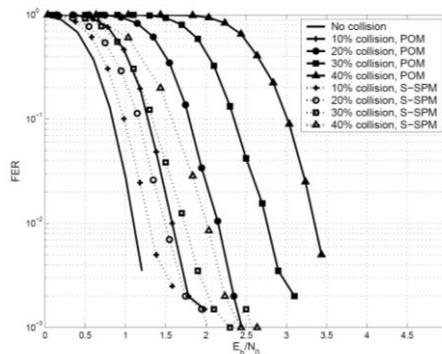
**Fig. 3.** FER performance comparison of POM and S-SPM
